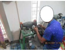
Nc picture 2: Grinding machine operator was not using hand gloves during work.
