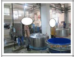
Nc picture 4: Hydro extractor machine operators were not using hand gloves.
